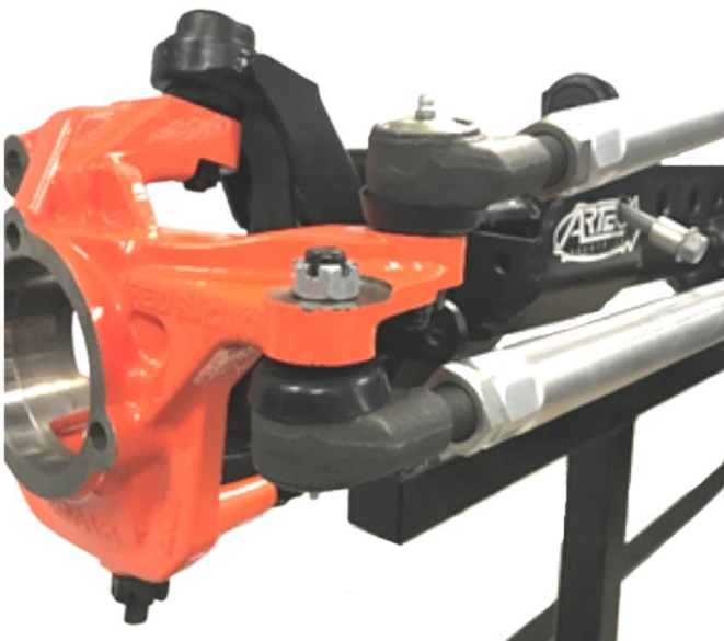
Over Knuckle Flip Drag Link and Tie Rod
